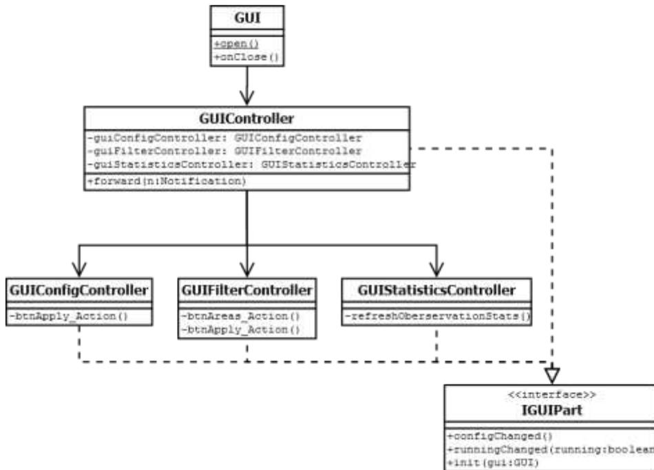
Each controller implements the Interface IGUIPart, which unifies calls and communication. It consists of:
