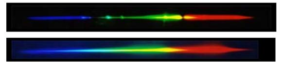
**Figure 6.** *Above.* Spectrum of a sodium lamp. At least six emission lines and one absorption line can be very well resolved. *Below.* Spectrum of a car-light.
