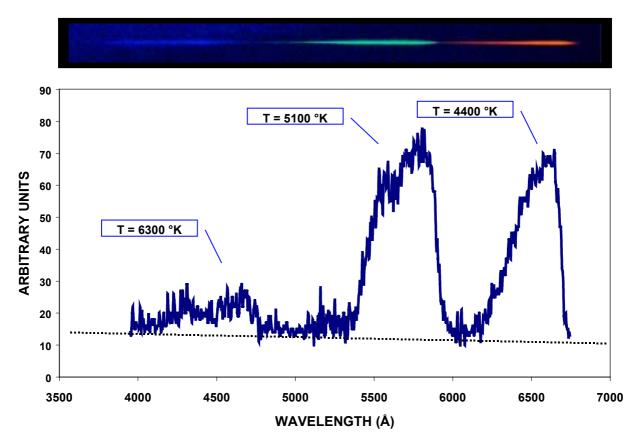
**Figure 7.** Spectrum of a Hessdalen light-phenomenon obtained with a ROS grating in connection with a Praktica BX-20 reflex camera equipped with a 270 mm lens. The dotted line indicates the level of noise. The three peaks are indicated with the relative temperatures which are derived from the Wien law. The wavelength range in which the spectrum is detected responds to the sensitivity curve of a Kodak Ektachrome 100 film [12], which was used to take the spectrum.
